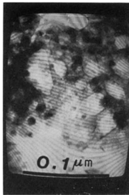
Figure 13 Electron micrograph of \text{Ni}_{66}\text{B}_{34} layer annealed at 500^\circ\text{C} for 5 h.
